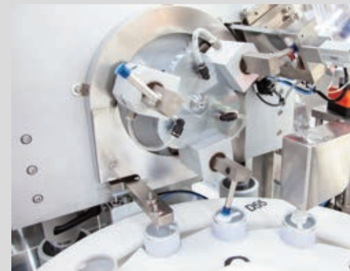
• Three-Head rotary spoon pick and place mechanism feeder
