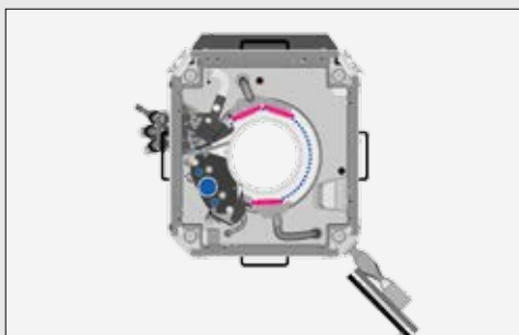
Mono-layer tablet production with 3 compression stations
