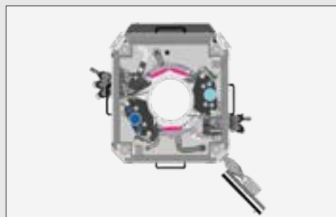
Bi-layer tablet production with tamping, pre-pressure and main pressure stations
