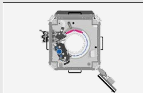
Mono-layer tablet production with 2 compression stations
